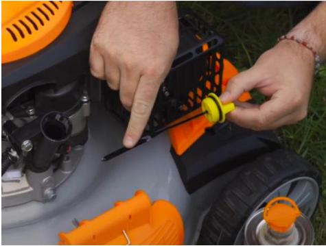
Change the engine oil after the first 5 hours of operation, this being the running-in period, then every 25 hours of operation or every 6 months.
