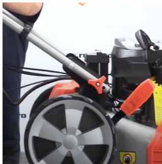
2. Install the control handle with the quick-setting clamps.
