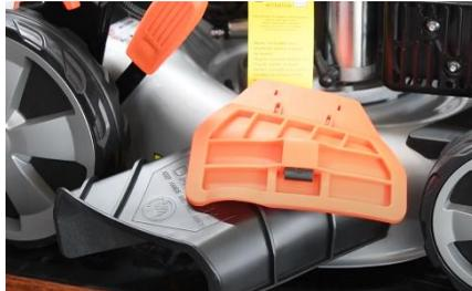
2. Lock the exhaust hole with the cover to activate the mulching and lateral evacuation function.
